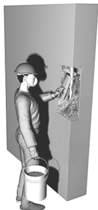
Fig. 8—Hand application of repair material.
