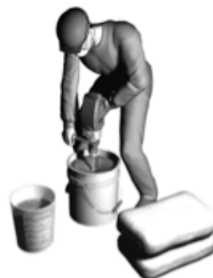
Fig. 7—Typical equipment to mix materials.
